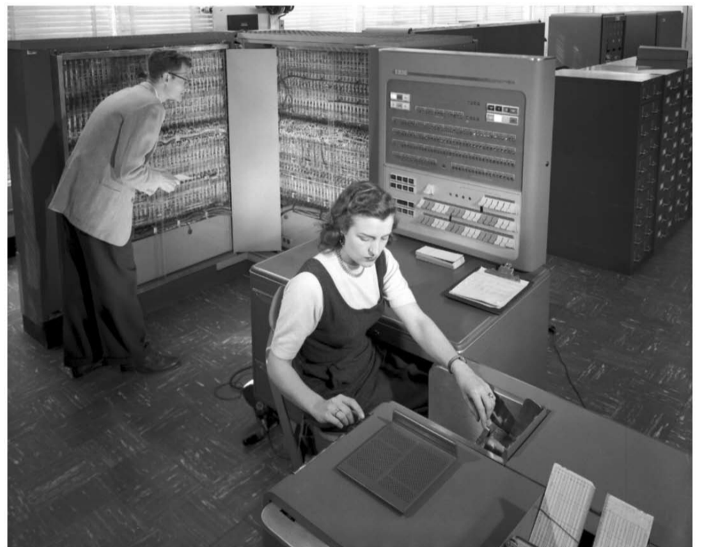
abb. dialektik der aufklärung 2 : a IBM 704, 1st mass produced computer with floating point arithmetic hardware, sings Daisy Bell at Bell Laboratories, murray hill NJ, 1961
